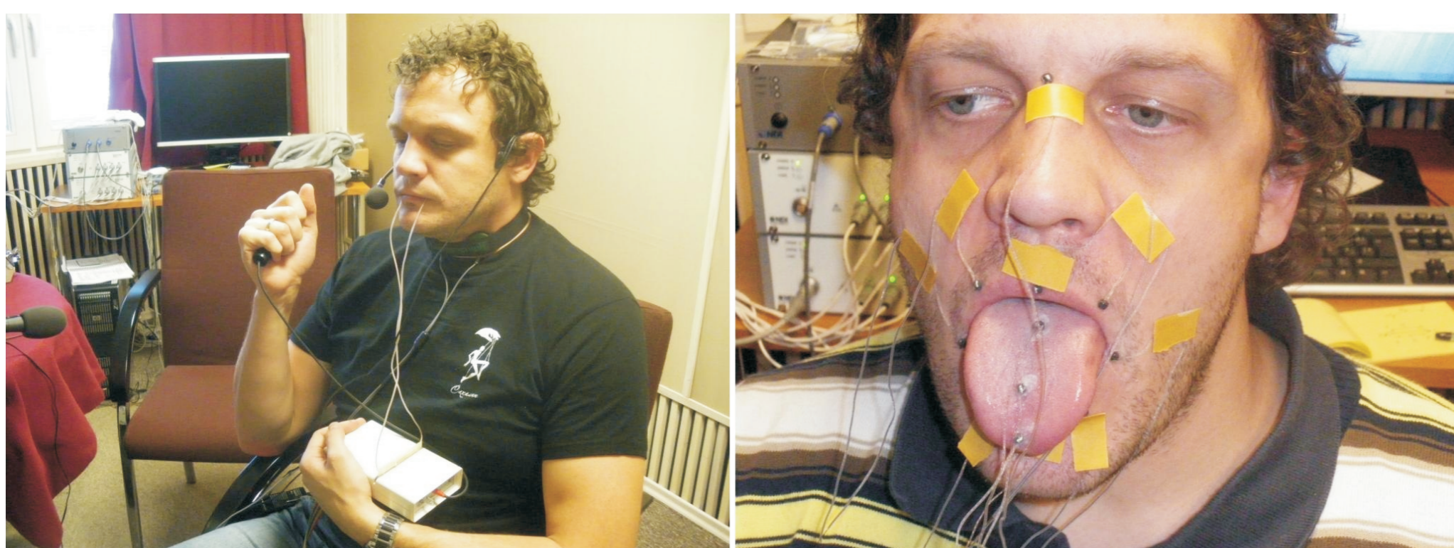
Figure 2. Left: the subject wearing electrodes of the EGG system, the EPG palate, and a close-talking microphone in the recording set-up 1; right: the position of EMA electrodes in the recording set-up 2.
